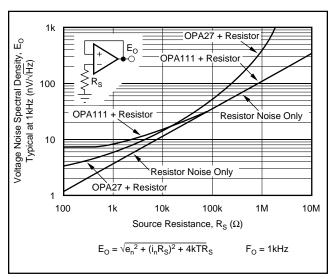
FIGURE 5. Voltage Noise Spectral Density Versus Source Resistance.
