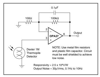
FIGURE 14. Long-Wavelength Infrared Detector Amplifier.
