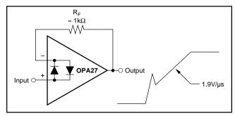
FIGURE 6. Pulsed Operation.
