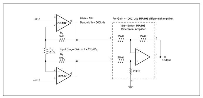
FIGURE 12. Low Noise Instrumentation Amplifier.
