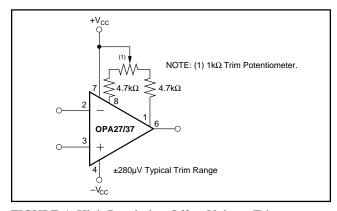
FIGURE 4. High Resolution Offset Voltage Trim.
