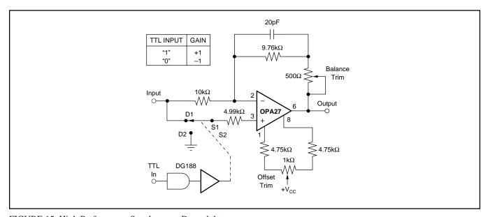
FIGURE 15. High Performance Synchronous Demodulator.
