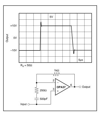
FIGURE 18. High Slew Rate Unity-Gain Buffer.
