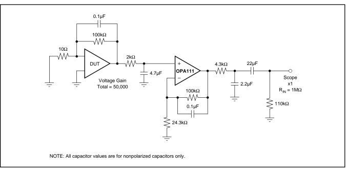
FIGURE 1. 0.1Hz to 10Hz Noise Test Circuit.
