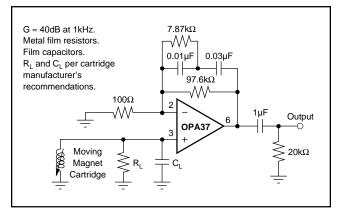
FIGURE 7. Low-Noise RIAA Preamplifier.
