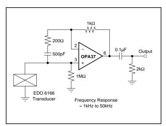
FIGURE 13. Hydrophone Preamplifier.
