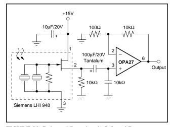
FIGURE 20. Balanced Pyroelectric Infrared Detector.
