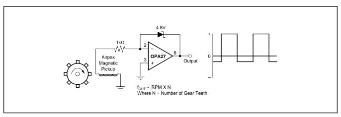
FIGURE 21. Magnetic Tachometer.
