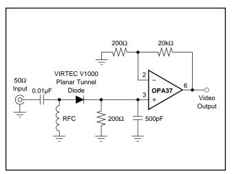
FIGURE 19. RF Detector and Video Amplifier.
