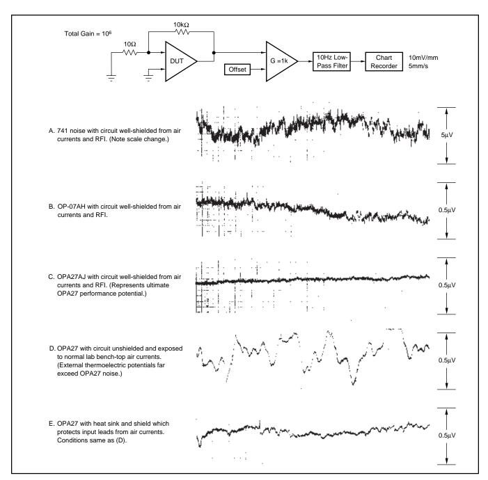
FIGURE 11. Low Frequency Noise Comparison.
