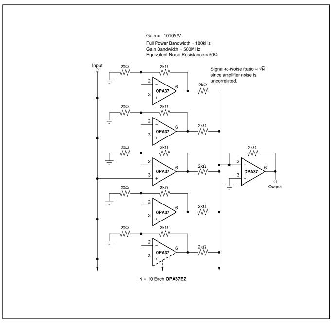
FIGURE 16. Ultra-Low Noise "N"-Stage Parallel Amplifier.
