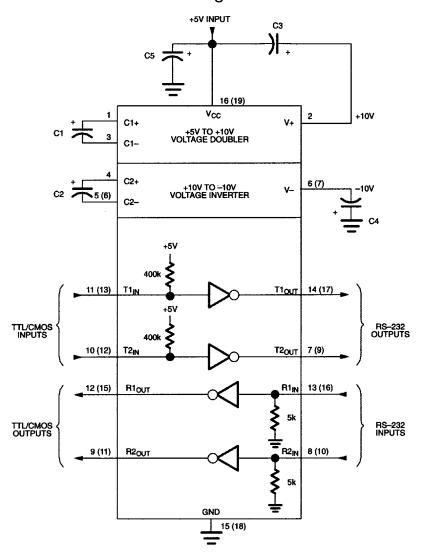
NOTE: C5 is a recommended decoupling capacitor which is the same value as C1, C2, C3, and C4.
