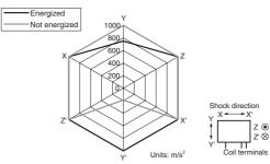
Measurement conditions: Impose a shock in the  $\pm X$ ,  $\pm Y$ , and  $\pm Z$  directions three times each with the Relay energized to check the shock values that cause the Relay to malfunction.
