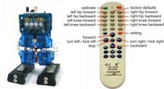
Using the remote you can make the robot walk forward, backward, turn left or right or stop and kick with either the left or right foot. As the center position of servos can change with temperature, the servos can be calibrated using the remote. New positions are automatically saved in EEPROM.
