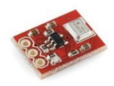
Ready to add sound detection to your next project? This small breakout board from SparkFun couples a tiny microelectromechanical system (MEMS) microphone with a 67x gain external amplifying circuit, converting sound into analog voltage signals that can be measured by a microcontroller's analog-to-digital converter (ADC). The unit comes fully assembled as shown and works from 1.5 to 3.3 V.
