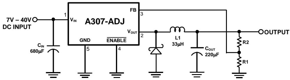
$$V_{OUT} = V_{REF} \left( 1 + \frac{R2}{R1} \right)$$
