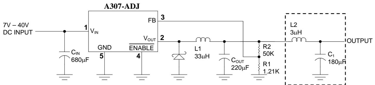
**Figure 4. LC Filter for Low Output Ripple**
