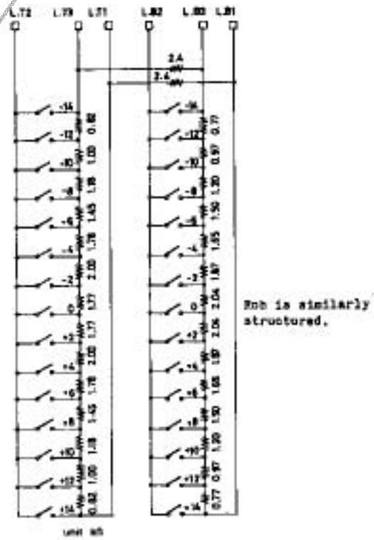
When data of -00 is transferred to main volume control 1dB STEP, S1,S2 are brought to open state and S3,S4 are turned ON simultaneously.
