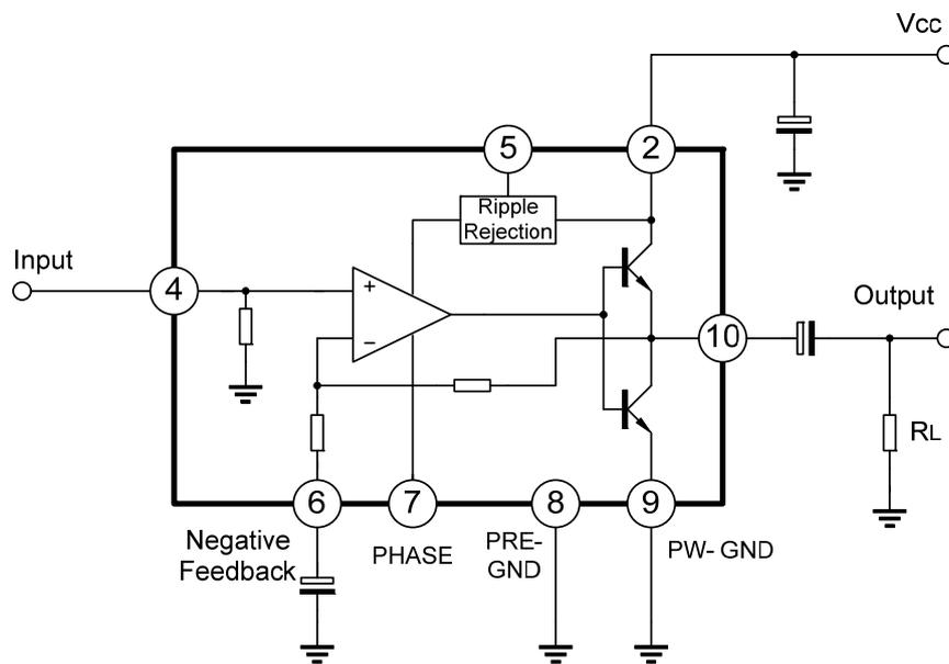
Note: Pin connection for SSOP-10 package only.
