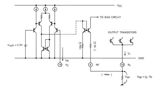
Negative Feedback is looped by RF and connected its line to pin (8). Feedback Voltage  $V_{NF}$  is generated by RF and Output Current IO. It is possible to decrease the feedback by connecting a resistor between pin (10) and pin (8). Input current of  $V_{C}$  (IC IN) vs  $V_{C}$  characteristic is shown below.
