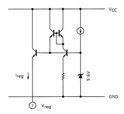
Internal regulator outputs 5 V and this current capability is up to 30 mA.  $V_{\rm CC}$  vs  $V_{\rm reg}$  characteristic is shown below.
