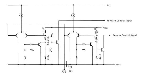
FRS input is a control terminal of Motor Rotation Direction and Stop.  $V_{\rm FRS}$  vs IFRS characteristic is shown below.
