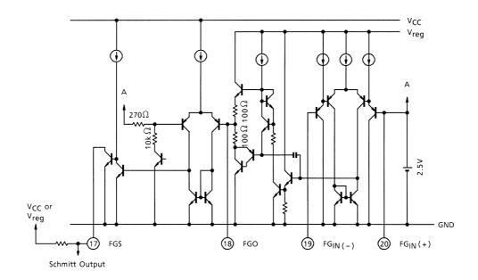
2.5~V of Internal Reference is equipped with FG Amplifier. FG signal is fed into FGIN + and FGIN - inputs with differential mode and outputs to FGO (Pin (18)).
