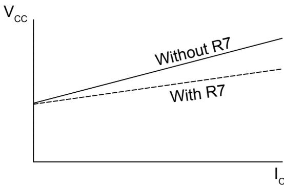
Figure 5. V<sub>CC</sub> versus I<sub>O</sub> (secondary load)
