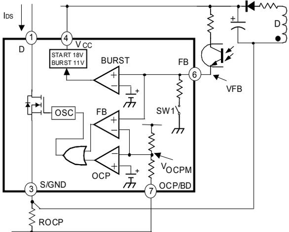
Figure 14. REG circuit functional block diagram
