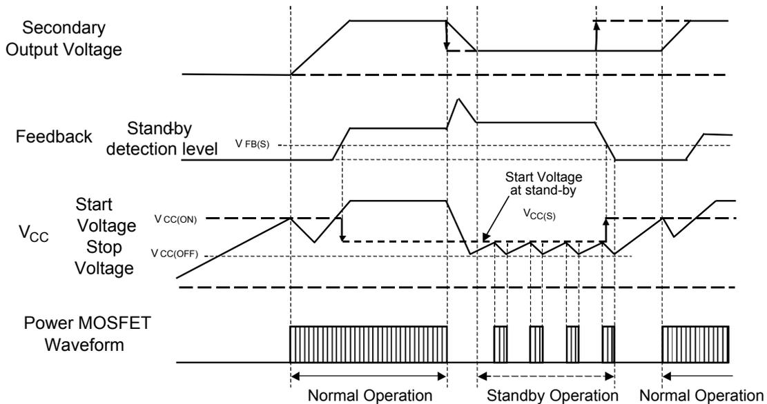
Figure 19. Quasi-resonant to bottom-skip operation timing
