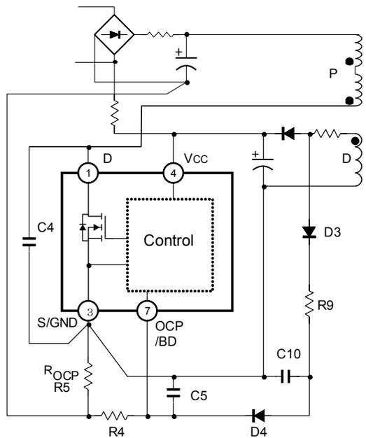
Figure 16. Quasi-resonant and delay circuit
