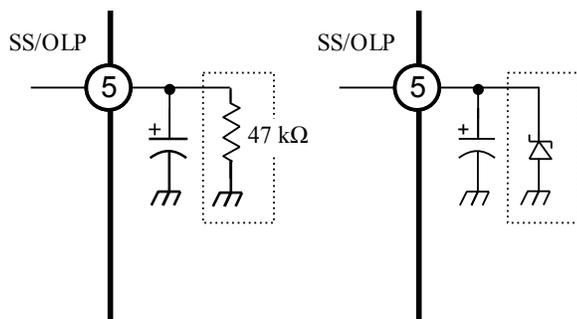
Figure 12. OLP deactivation circuit alternative configurations
