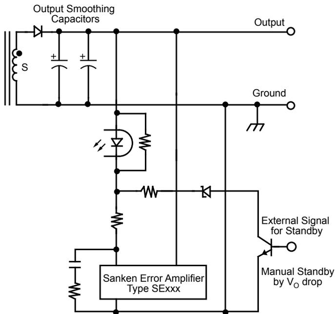
Figure 24. Output circuit
