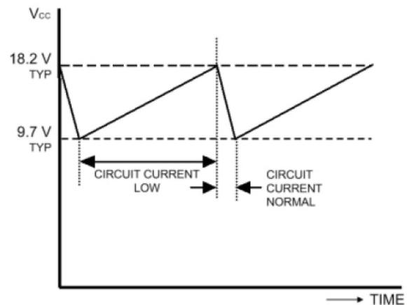
Figure 7. V<sub>CC</sub> during latch mode
