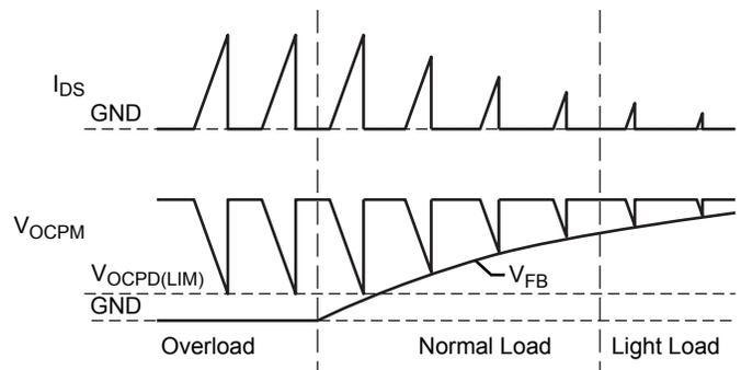
Figure 13. Constant-voltage control at fixed oscillation frequency (quasi-resonant signal not available)
