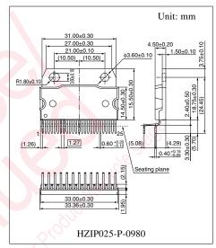
Note) The package of this product will be changed to lead-free type (HZIP025-P-0980B). See the new package dimensions section later of this detector.
