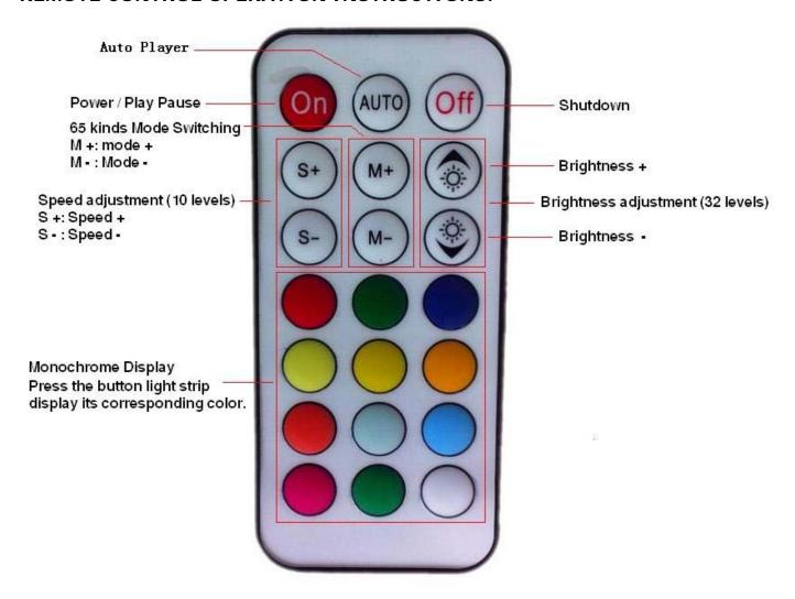
**Note:** The boot state press the "On" button to pause playback, press again the "On" button can resume playing.
