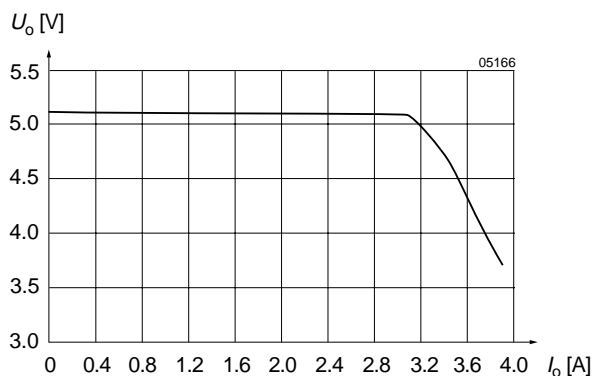
Fig. 9 U_o versus I_o (typ) of units with U_o = 5.1 V. (110 IMY 15-05-7R)
