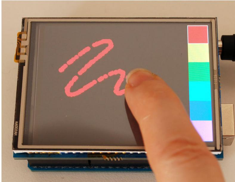
Spice up your Arduino project with a beautiful large touchscreen display shield with built in microSD card connection. This TFT display is big (2.8" diagonal) bright (4 white-LED backlight) and colorful (18-bit 262,000 different shades)! 240x320 pixels with individual pixel control. It has way more resolution than a black and white 128x64 display. As a bonus, this display has a resistive touchscreen attached to it already, so you can detect finger presses anywhere on the screen.
