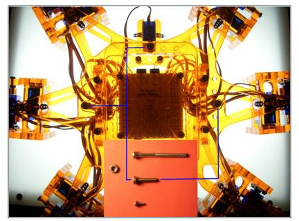
Lastly, use 3 pairs of medium screws and nuts to secure the battery shelf (X-shaped plate) to the underside of your robot.
