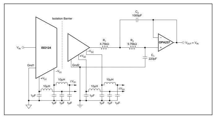
FIGURE 4. Optional π Filter to Minimize Power-Supply Feedthrough Noise; Output Filter to Remove 500kHz Carrier Ripple. For more information concerning output filters refer to Application Notes SBPA012 and SBFA001.
