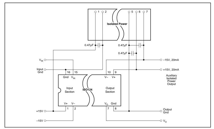
FIGURE 11. Input-Side Powered ISO Amp.
