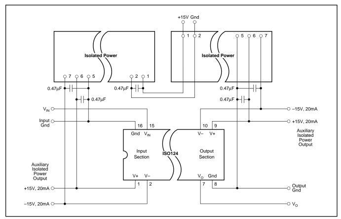
FIGURE 12. Powered ISO Amp with Three-Port Isolation.
