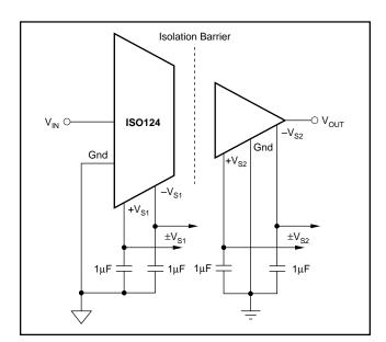
FIGURE 2. Basic Signal and Power Connections.
