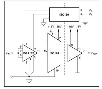
FIGURE 3. Programmable-Gain Isolation Channel with Gains of 1, 10, and 100.
