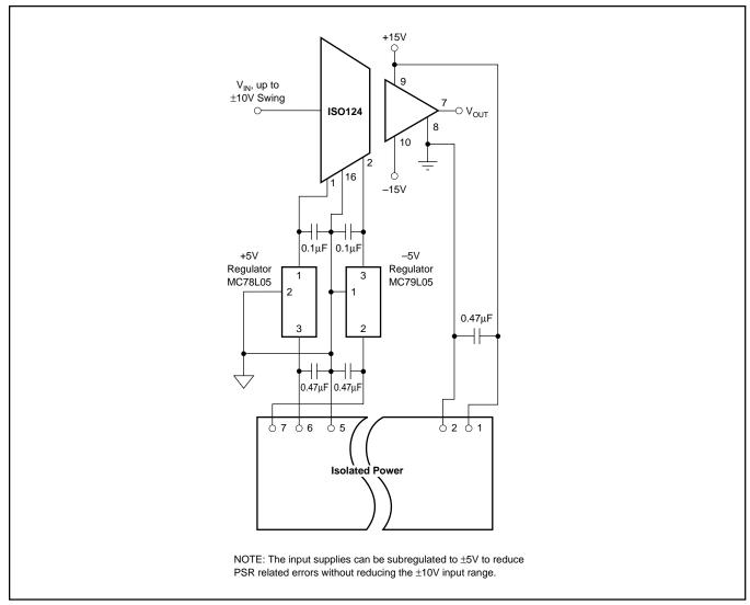
FIGURE 9. Improved PSR Using External Regulator.
