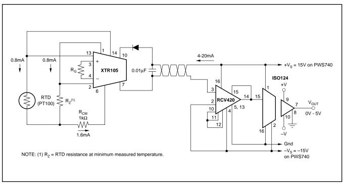
FIGURE 7. Isolated 4-20mA Instrument Loop. (RTD shown.)
