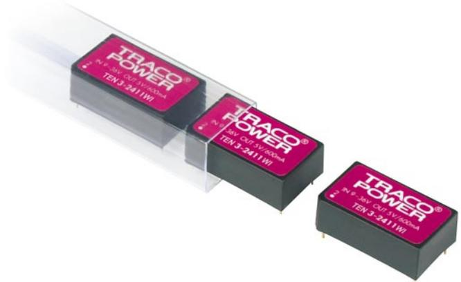
The TEN 3WI series is a family of dc-dc converter modules with 3W output power, featuring ultra wide 4:1 input voltage ranges of 9-36VDC or 18-75VDC. They come in a DIP-24 plastic package with industry-standard footprint. A high efficiency up to 84% allows operation ambient temperatures of -40°C to +70°C at full load.
