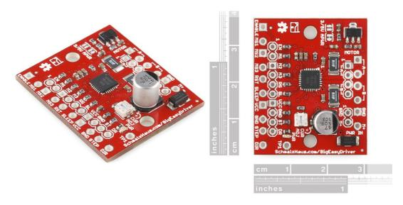
**Description:** The Big Easy Driver, designed by <u>Brian Schmalz</u>, is a stepper motor driver board for bi-polar stepper motors up to 2A/phase. It is based on the Allegro A4983 stepper driver chip. It's the next version of the popular Easy Driver board.
