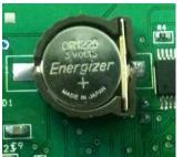
First Install battery for RTC , " + " mark on top RTC DS1307 - 68 in i2cdetect –y 0 or i2cdetect –y 1 for Rs-Pi V2 you will see 68 in the screen 68 -> RTC DS1307 48 -> tmp102
