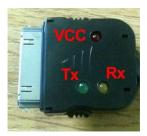
3 LED for indicate the states of the cable DC 3.3V (Red) , Tx (Green) , Rx (Yellow)
