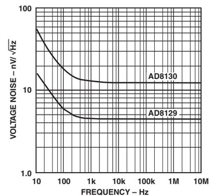
TPC 63. AD8129/AD8130 Input Voltage Noise vs. Frequency
