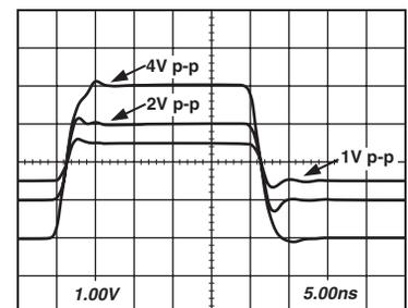
TPC 81. AD8130 Transient Response vs. Output Amplitude,  $V_{OUT} = 1\text{ V p-p}$ ,  $2\text{ V p-p}$ ,  $4\text{ V p-p}$
