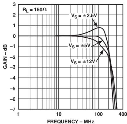
TPC 7. AD8130 Frequency Response vs. Supply,  $R_L = 150\ \Omega$
