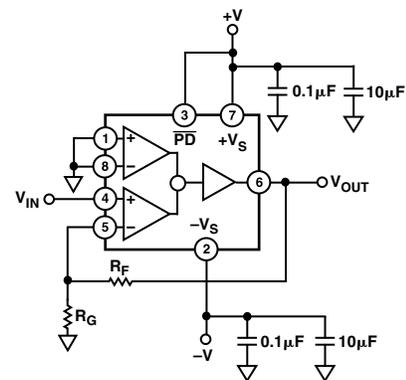
*Figure 4. With both inputs grounded, the feedback stage functions like an op amp:  $V_{OUT} = V_{IN} (1 + R_F/R_G)$ . NOTE: This circuit is provided to demonstrate device operation. It is not suggested to use this circuit in place of an op amp.*
