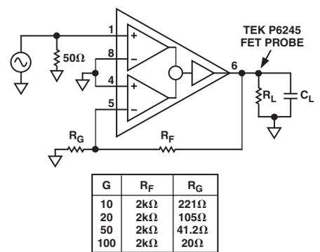
TPC 36. AD8129 Basic Frequency Response Test Circuit
