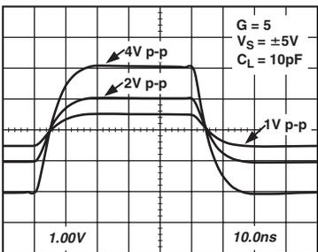
TPC 88. AD8130 Transient Response vs. Output Amplitude
