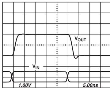
TPC 86. AD8130 Transient Response with  $-3\text{ V}$  Common-Mode Input
