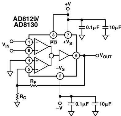
Figure 5. Basic Gain Circuit:  $V_{OUT} = V_{IN} (1 + R_F/R_G)$
