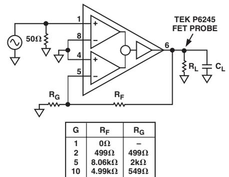
TPC 18. AD8130 Basic Frequency Response Test Circuit
