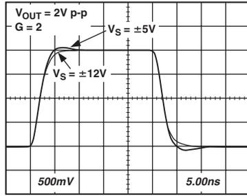
TPC 83. AD8130 Transient Response vs. Supply,  $V_{OUT} = 2\text{ V p-p}$ ,  $G = 2$
