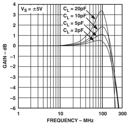
TPC 22. AD8129 Frequency Response vs. Load Capacitance
