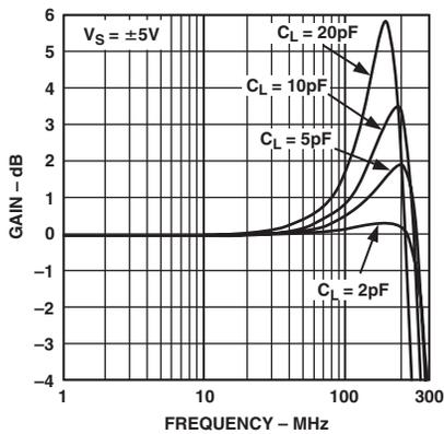
TPC 4. AD8130 Frequency Response vs. Load Capacitance
