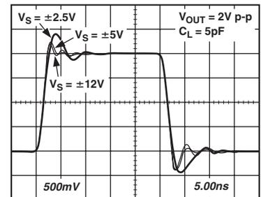
TPC 78. AD8130 Transient Response vs. Supply,  $V_{OUT} = 2\text{ V p-p}$ ,  $C_L = 5\text{ pF}$
