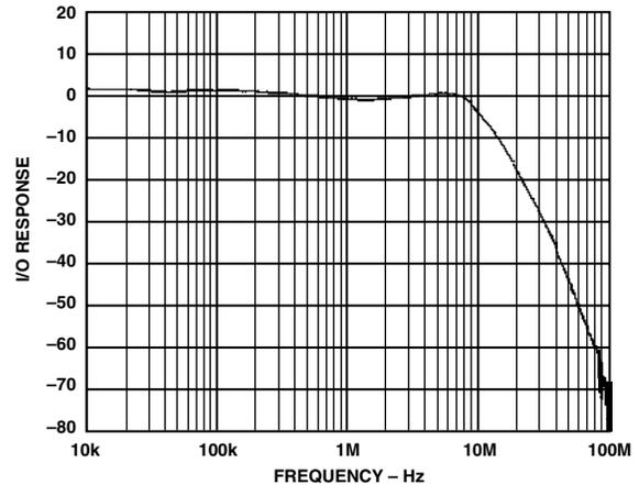
Figure 10. Combined Response of Cable Plus Equalizer
