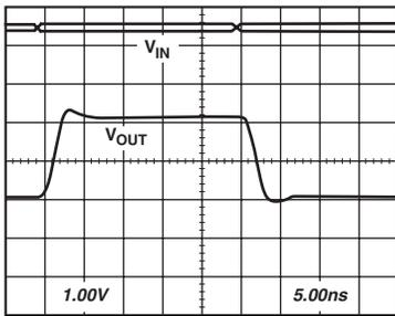
TPC 103. AD8129 Transient Response with  $+3.5\text{ V Common-Mode Input}$
