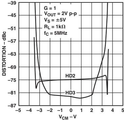
TPC 55. AD8130 Harmonic Distortion vs. Common-Mode Voltage
