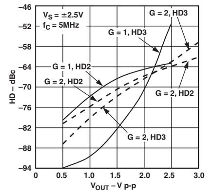
TPC 45. AD8130 Harmonic Distortion vs. Output Voltage
