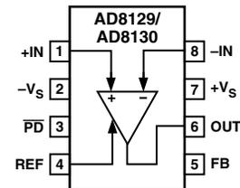
data transmission. The AD8129 and AD8130 are differential-to-single-ended amplifiers with extremely high CMRR at high frequency. Therefore, they can also be effectively used as high-speed instrumentation amps or for converting differential signals to single-ended signals.
