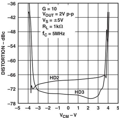
TPC 58. AD8129 Harmonic Distortion vs. Common-Mode Voltage
