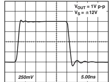
TPC 75. AD8130 Transient Response,  $V_S = \pm 12\text{ V}$ ,  $V_{OUT} = 1\text{ V p-p}$
