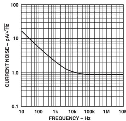
TPC 62. AD8129/AD8130 Input Current Noise vs. Frequency
