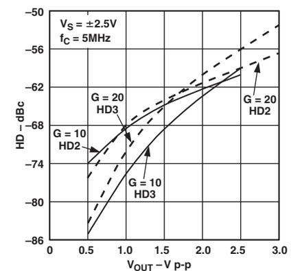
TPC 54. AD8129 Harmonic Distortion vs. Output Voltage
