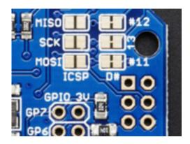
If you're using a Mega or Leonardo Arduino, you'll need to short the jumpers on the top right of the board, and install the 2x3 socket header. This is because those Arduinos use the 2x3 pin header for the hardware-SPI pins and hardware-SPI is required for the high-speed data transfer required by the VS1053 codec. We'll cover that in the Assembly step.
