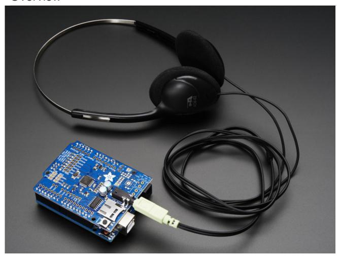
Bend all audio files to your will with the Adafruit Music Maker shield for Arduino! This powerful shield features the VS1053, an encoding/decoding (codec) chip that can decode a wide variety of audio formats such as MP3, AAC, Ogg Vorbis, WMA, MIDI, FLAC, WAV (PCM and ADPCM). It can also be used to record audio in both PCM (WAV) and compressed Ogg Vorbis. You can do all sorts of stuff with the audio as well such as adjusting bass, treble, and volume digitally.
