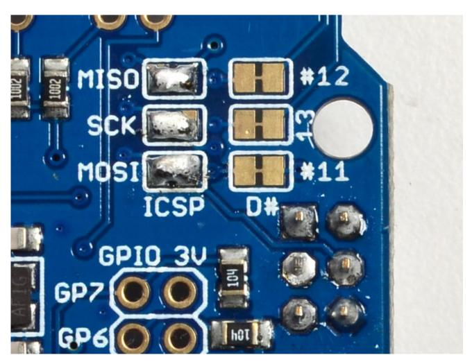
You can also cut the mini wire between the other three jumpers to 'release' the digital #11, 12 and
