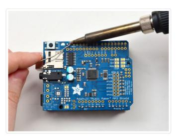
Don't forget the 6-pin socket!
