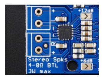
In the bottom left is an amplifier section, this is a stereo 3W amplifier, with bridge-tied load output. It's only meant for driving speakers directly! Do not connect to another amplifier, use the line out for that! Also, you cannot bridge-tie R and L together - if you need only one speaker, leave the unused one disconnected.
