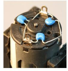
But my motor already has a capacitor on it and it still doesn't work. These motors generate a lot of brush noise and usually need the full 3-capacitor treatment for adequate suppression. These motors generate a lot of brush noise and usually need the full 3-capacitor treatment for adequate suppression.
