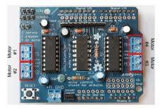
**Note:** Higher frequencies will produce less audible hum in operation, but may result in lower torque with some motors.
