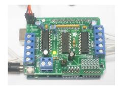
Arduino is a great starting point for electronics, and with a motor shield it can also be a nice tidy platform for robotics and mechatronics. Here is a design for a full-featured motor shield that will be able to power many simple to medium-complexity projects.
