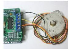
Stepper motors are great for (semi-)precise control, perfect for many robot and CNC projects. This motor shield supports up to 2 stepper motors. The library works identically for bi-polar and uni-polar motors
