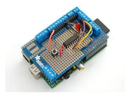
Now that you've finally got your hands on a Raspberry Pi® (http://adafru.it/aHx), you're probably itching to make some fun embedded computer projects with it. What you need is an add on prototyping Pi Plate from Adafruit, which can snap onto the Pi main board assembly (and is removable later if you wish) and gives you all sorts of prototyping goodness to make building on top of the Pi super easy.
