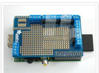
This part is optional, but if you want to have sockets for the GPIO pins so you can plug wires in and out easily, you can solder in the two 8-pin and single 6-pin header.
