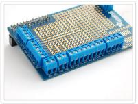
Place the blue terminal blocks around the perimeter of the Proto Plate PCB. Make sure you place them so that the open ends are facing out as shown.
