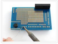
Solder each terminal block connection to the PCB using plenty of solder to make a strong mechanical connection
