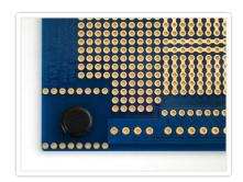
Place the single bumper underneath the SOIC breakout area. This will make the plate sit nicely on the Ethernet port
