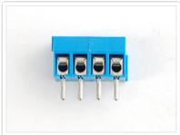
Find the terminal blocks, they're blue and come in 3-pin and 2-pin shapes. We'll need to slide the blocks together for the next step where we put the blocks into the proto plate. Slide them together to make 1x8 pin, 1x5 pin, and 3x4pin terminal blocks
