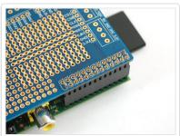
Heat up the soldering iron to 650 °F and wait for it to get up to temperature. Then heat a corner pad/pin with the iron tip and after two seconds poke in a small amount of solder. After the solder has melted into the pad/pin remove the iron.
