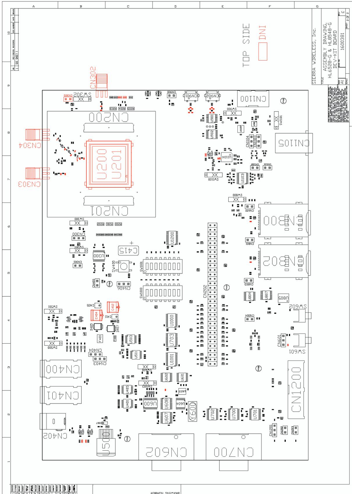
Figure 2. Available Connectors and Components on the AirPrime HL Series Development Kit
