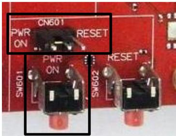
Figure 8. PWR ON Pushbutton and CN601 Jumper
