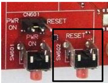
Figure 9. ~RESET Pushbutton
