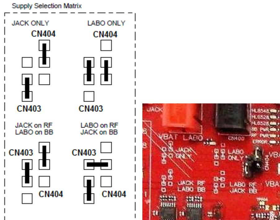
Figure 7. Power Source Selection (schematic diagram and actual development kit picture)
