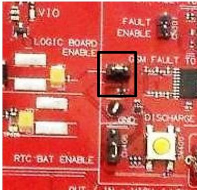
Figure 15. Jumper for Supplying the Development Kit Interfaces Separately
