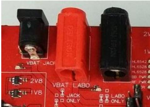
Figure 6. Power Supply Connector (CN402, CN401 and CN400)
