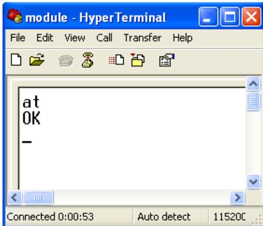
Figure 19. Communicating with the AirPrime HL6528x
