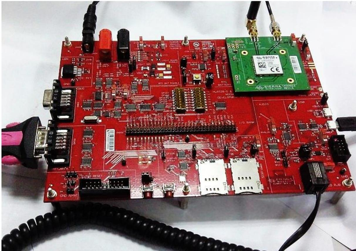
Figure 16. AirPrime HL Series Development Kit (with an HL6528x Socket Board and HL6528 Embedded Module)
