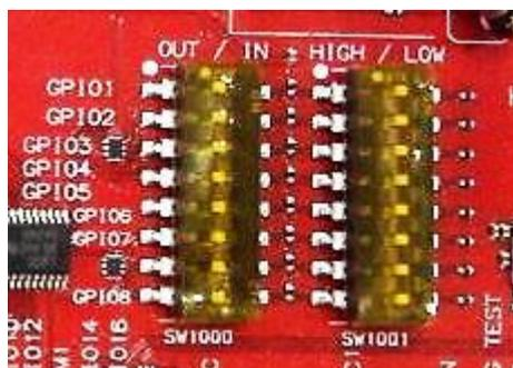
Figure 14. GPIOs Control Switches
