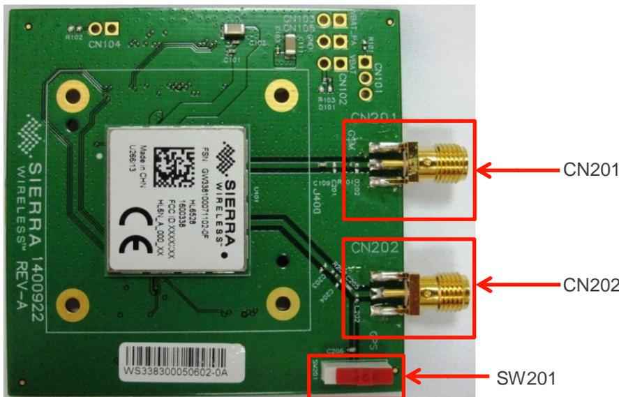
Figure 3. AirPrime HL6528x Socket Board (with an HL6528 embedded module)
