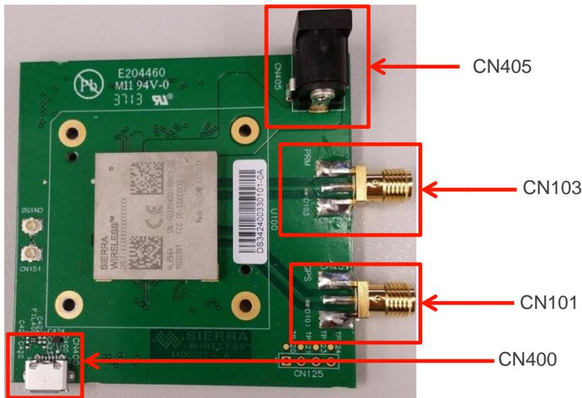
Figure 4. AirPrime HL8548x Socket Board (with an HL8548 embedded module)
