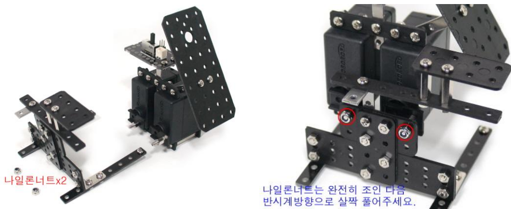
12. Fix the support which conneted to motor guide and option frame of leg part with nylon nut
