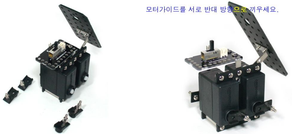
11. Insert the motor guide to DC motor axle. In this case, inserting the motor guide in opposite directions
