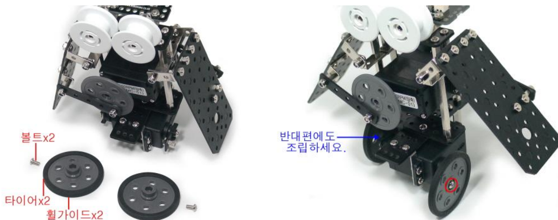
18. Put the Wheel-guide into the tire and fix them on the 5mm Supports which is fixed to the Motor guides with bolts.
