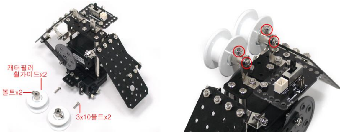
16. Put the L2x2 Frames to the 3x10bolts and the Caterpillar Wheel-guide to the 3x10bolts. Fix the Caterpillar Wheel-guide with bolts not to move.
