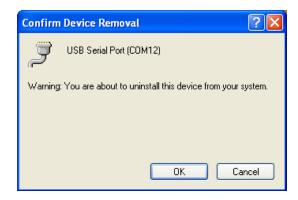
After you have uninstalled ARM-USB-OCD-H drivers from Device Manager, disconnect the programmer from your computer.
