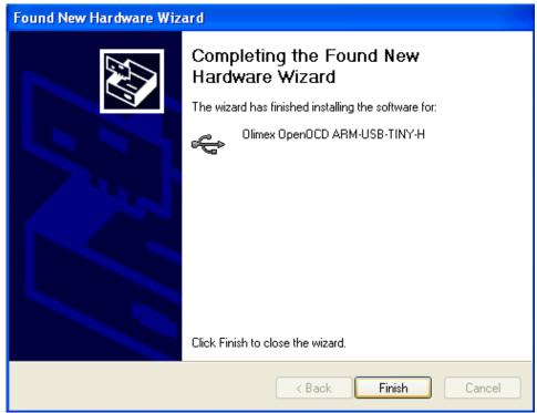
When this window appears – press "Finish". Windows will ask you again for drivers and you should repeat the same procedure with the same drivers. After the second installation of your drivers – check in Device Manager for your new device:
