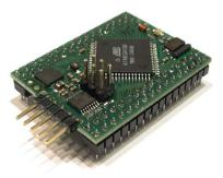
A preinstalled firmware (ATmegaBOOT) provides an SKT500 compatible bootloader, hence no ISP adapter is required for programming the ATmega128. A serial crossover cable connects the serial port to a PC running the programming software (e.g. AVR-Studio, uisp, avrdude, etc.). ATmegaBOOT can also be used for low level hardware tests of the ATmega128 microcontroller and peripheral circuits.
