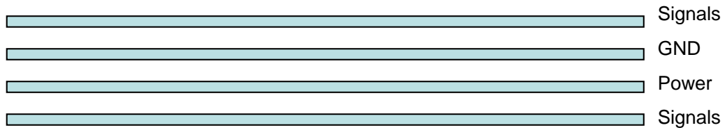
Figure 17: Typical 4-layer PCB construction
