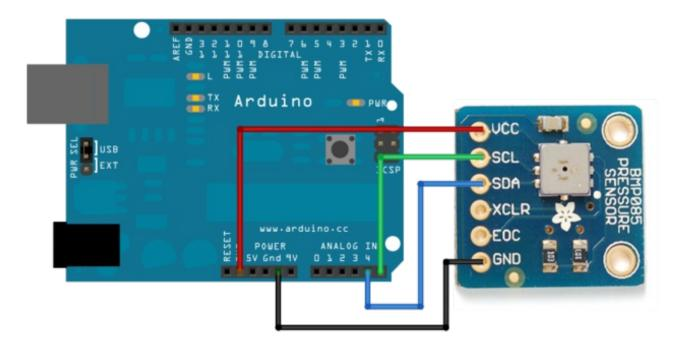
Connect the **VCC** pin to a **3.3V** power source. The V1 of the sensor breakout cannot be used with anything higher than 3.3V so don't use a 5V supply! V2 of the sensor board has a 3.3V regulator so you can connect it to either 3.3V or 5V if you do not have 3V available.
