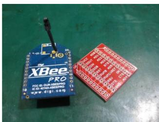
**Description:** This is a simple breakout board for the popular XBee product from Maxstream. This board breaks out all 20 pins of the XBee to a 0.1" standard spacing dual row header. The spacing between 0.1" headers is 0.5" making it breadboard DIP friendly. We highly recommend using the female sockets to avoid having to solder the XBee permanently to the breakout board. This is the PCB only. Please order the accompanying 2mm sockets (you'll need 2!) and 0.1" headers below.
