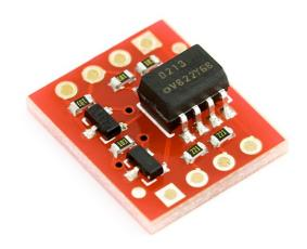
**Description:** This is a board designed for <u>opto-isolation</u>. This board is helpful for connecting digital systems (like a 5V microcontroller) to a high-voltage or noisy system. This board electrically isolates a controller from the high-power system by use of an opto-isolator IC. This IC has two LEDs and two photodiodes built-in. This allows the low-voltage side to control a high voltage side.
