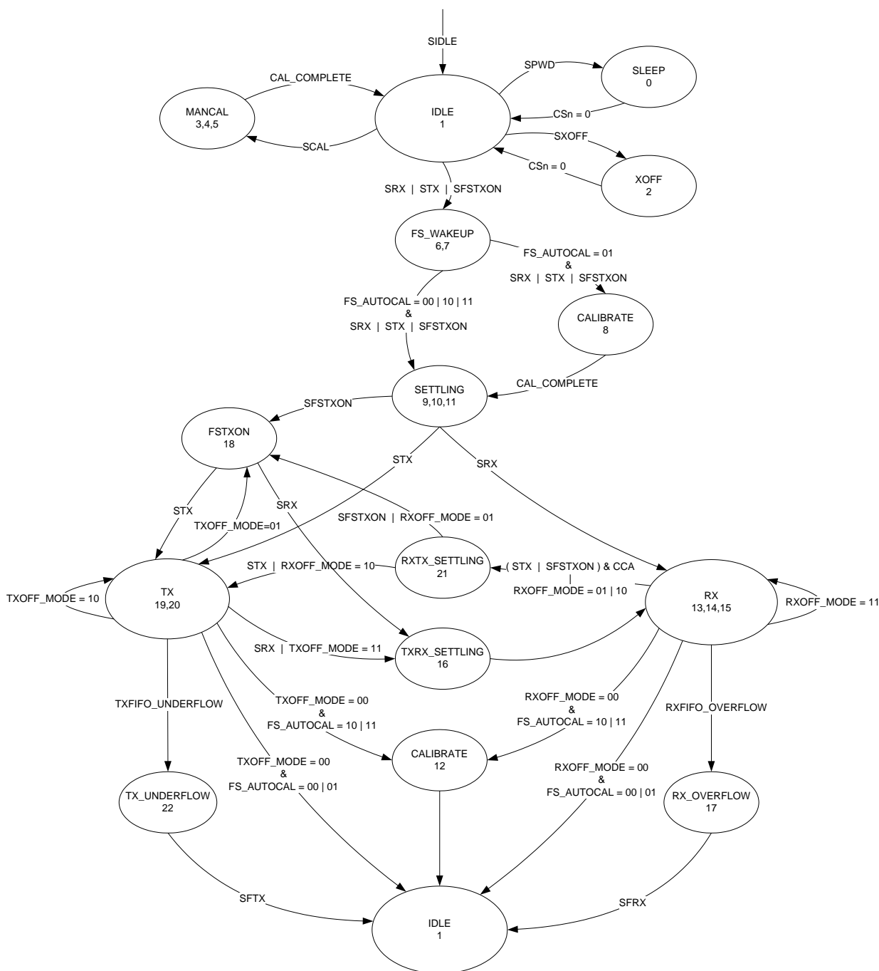
Figure 19: Complete Radio Control State Diagram
