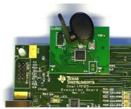
The CC2530EM, with the antenna mounted on the SMA connector, can be plugged into the SmartRF05EB.
