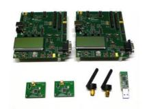
2 x CC2530EM 2 x 2.4 GHz Antennas 2 x SmartRF05EB 1 x CC2531 USB Dongle Batteries, cables and documentation
