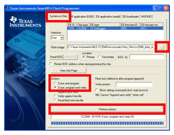
Select the appropriate flash image by clicking the browse button (marked "...") next to the flash image text field. You will find the flash images in <BLE stack install dir>\Accessories\Hex\_Files. Note that there are different files for the keyfob and the dongle.
