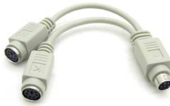
Figure 4-26 Y-Cable use for both Keyboard and Mouse
