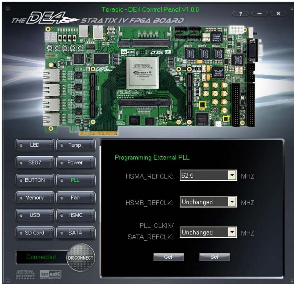
Figure 3–14 Programmable External PLL configured through Control Panel
