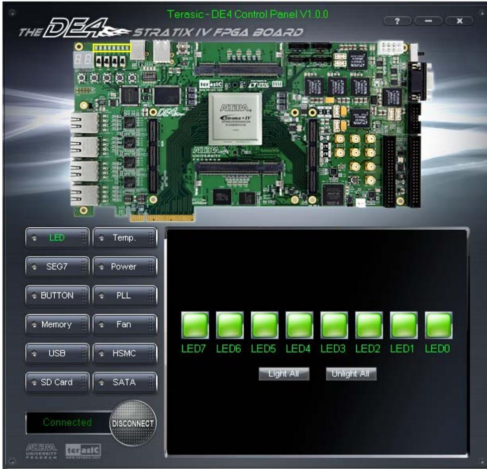
Figure 3–2 DE4 Control Panel is ready
