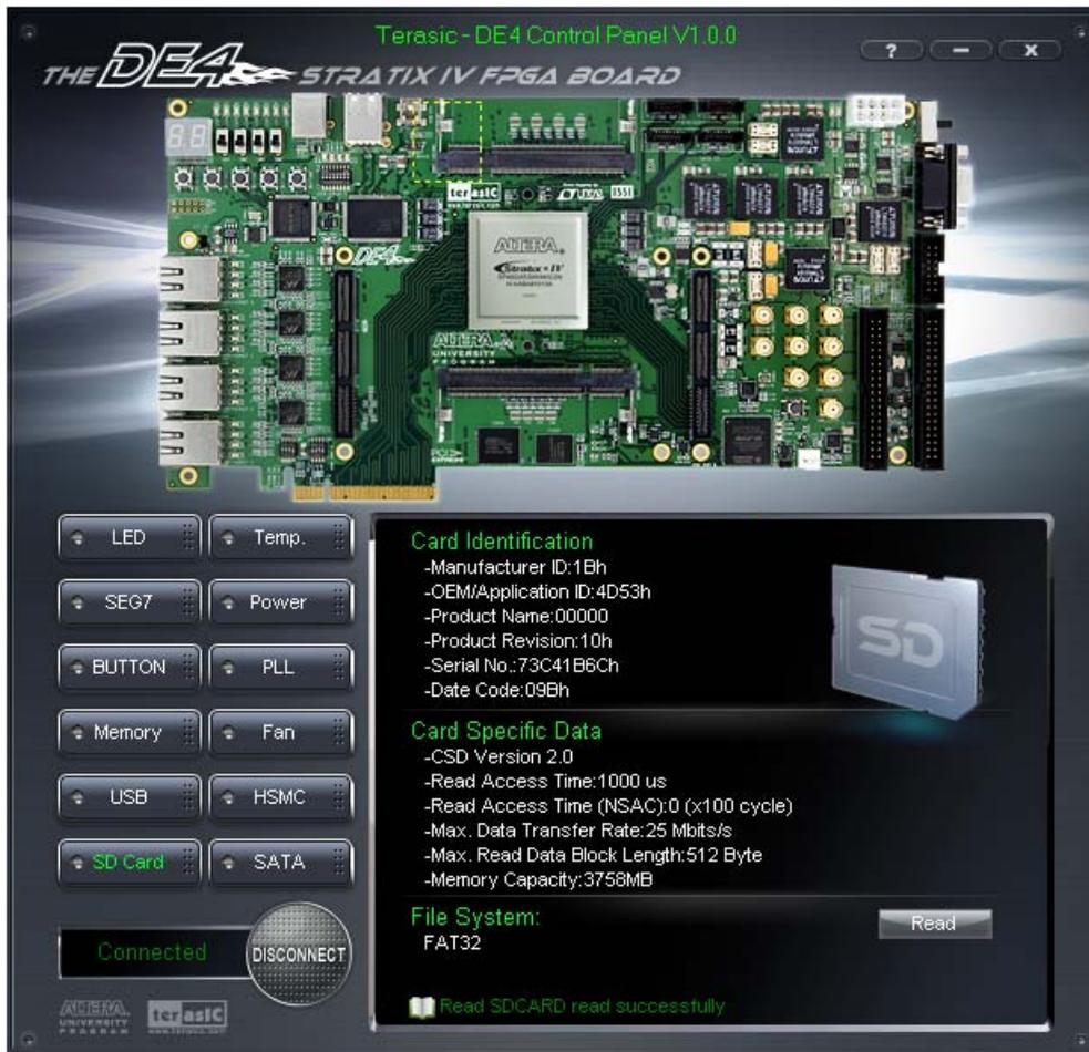
Figure 3–11 Reading the SD Card Identification and Specification
