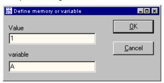
After confirming the dialog with OK, the Protocol Developer generates the code for this command. In the example this would be the code "MoveConst (A, 1);". This code can also be modified manually.
