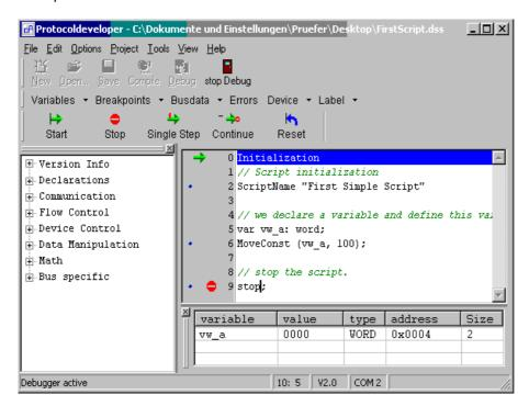
After you click onto the "continue" button the script is executed until a breakpoint is reached. The Debugger stops right before the breakpoint, so the stop command itself is not yet executed. Even in this case the variable window is refreshed.
