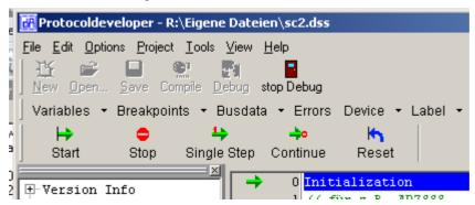
In our script we use a variable called vw\_a (our variable-naming convention for variable word, so we can see its type everywhere the variable is used). Now click on the variables button and add these variables to the window (right mouse "Add" in window or drop down list in variables button); thereafter it looks like this:
