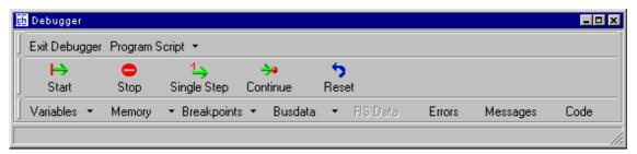
The main window of the Debugger enables to control a Gateway that is in the Debug Mode. The window offers the interface for operating and controlling the Debugger or the Debug Gateways.
