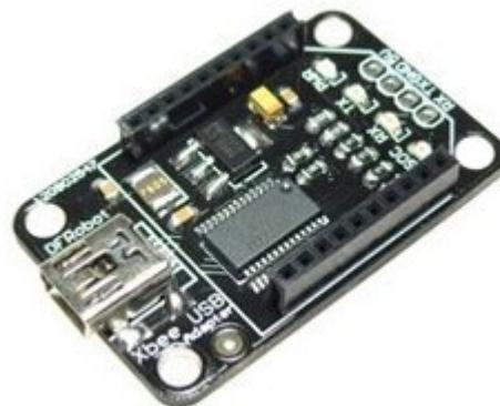
The *DFRobot Xbee USB adapter* is used for the XBee module configuration parameters to facilitate or to use as a wireless data transmission. It can be easily connected to a PC via mini USB cable. Further, it has XBee-setting support software X-CTU. It can also be used as a USB-TTL adapter.
