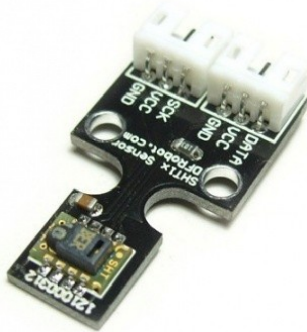
SHT1x Humidity and Temperature Sensor (SKU: DFR0066)
