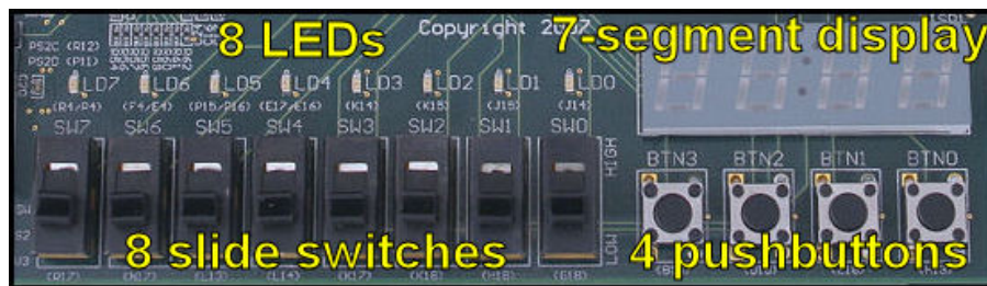
Figure 7: Nexys2 board I/O devices
