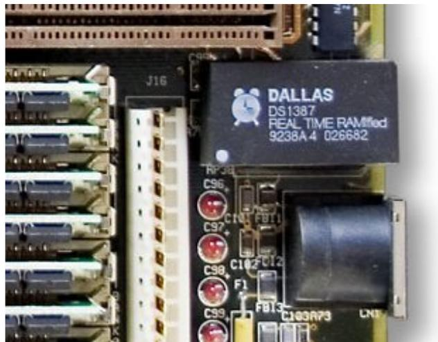
The image above shows a computer motherboard with a Real Time Clock called the **DS1387** (<http://adafru.it/aX0>). There's a lithium battery in there which is why it's so big.
