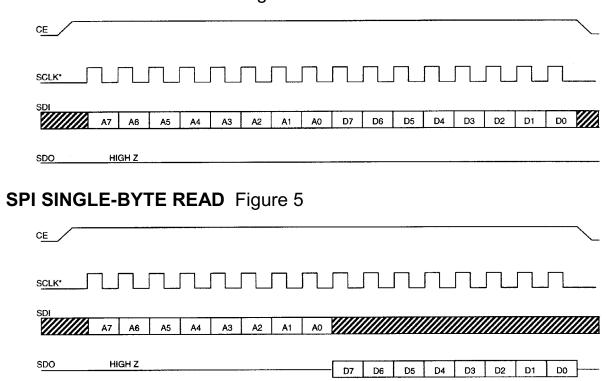
The address byte is always the first byte entered after CE is driven high. The most significant bit (A7) of this byte determines if a read or write will take place. If A7 is "0", one or more read cycles will occur. If A7 is "1", one or more write cycles will occur.
