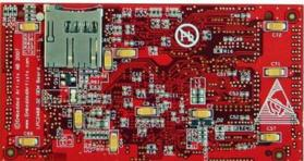
Embedded Artists' **LPC2468 OEM Board**, 32-bit databus, is equipped with NXP's **ARM7TDMI-S** based LPC2468 microcontroller suitable for multipurpose communication applications.
