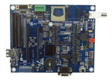
The LPCXpresso Base board makes it possible for you to get started with experiments and prototyping immediately. The Base board can also be used together with the **mbed** module.
