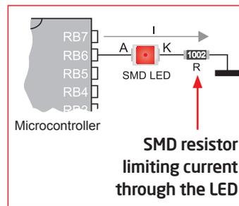
**LED (Light-Emitting Diode)** is a highly efficient electronic light source. When connecting LEDs, it is necessary to place a current limiting resistor so that LEDs are provided with the
