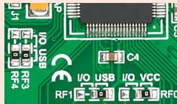
Microcontroller with USB support should be soldered to the MCU card with dedicated USB SMD jumpers. Make sure to solder **RF1**, **RF3** and **RF4** jumpers to USB position in order to connect USB lines to USB connector.
