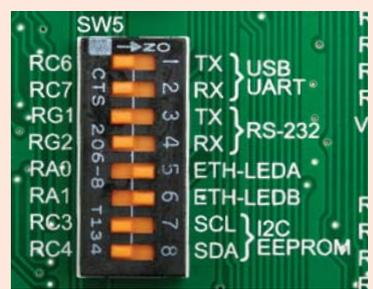
In order to enable ethernet LEDs, you must enable **SW5.5** (RA0) and **SW5.6** (RA1) DIP switches. This connects the **LEDA** and **LEDB** lines to appropriate microcontroller pins.
