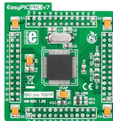
3 Figure 4-4: Standard 80-pin MCU card with **PIC18F8722**.
