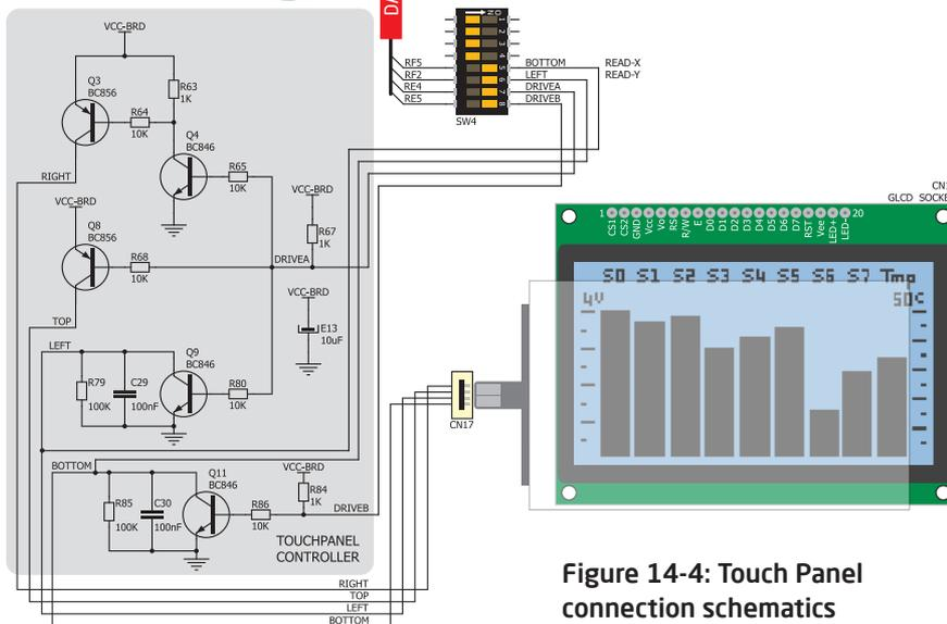
Figure 14-4: Touch Panel connection schematics
