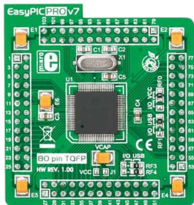
1 Figure 4-2: Standard 80-pin MCU card with **PIC18F87J50**, which supports USB.
