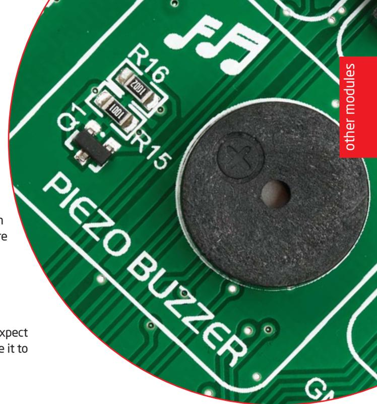
Figure 15-1: Piezo buzzer connected to RB6 microcontroller pin via SW4.4
