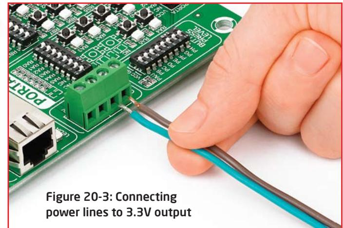
Figure 20-3: Connecting power lines to 3.3V output
