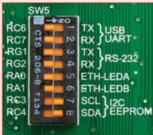
**Figure 19-1:** Activate SW5.7 and SW5.8 switches to enable pull-up resistors in I<sup>2</sup>C lines of Serial EEPROM.
