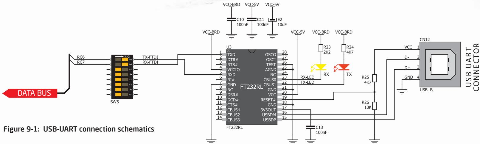
Figure 9-1: USB-UART connection schematics
