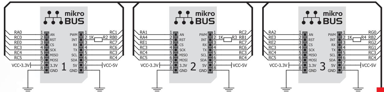
Figure 7-1: Connection schematics of on-board mikroBUS™ host sockets
