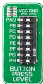
**Figure 6-5:** Button press level DIP switches (tri-state)
