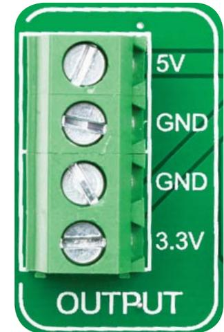
Figure 20-1: Output voltage terminals
