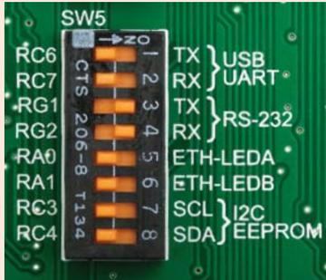
In order to enable RS-232 communication, you must push **SW5.3** (RG1) and **SW5.4** (RG2) to **ON** position. This connects the **RX** and **TX** lines to appropriate microcontroller pins and its second UART module.
