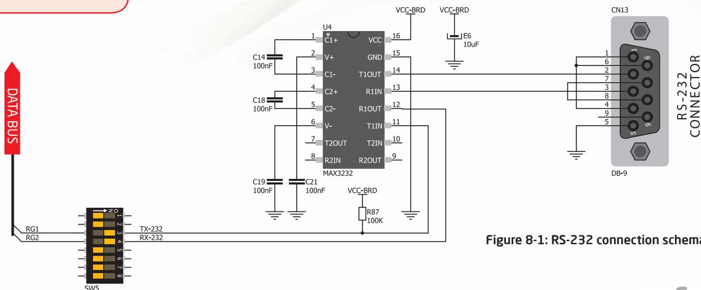
Figure 8-1: RS-232 connection schematics
