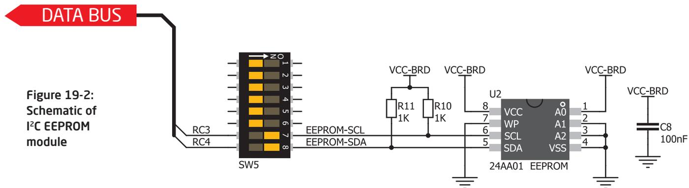
**Figure 19-2:** Schematic of I<sup>2</sup>C EEPROM module
