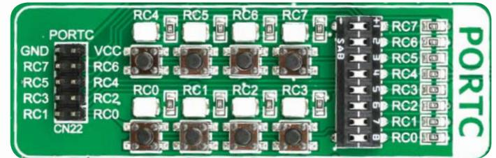
Figure 6-1: I/O group contains 3 PORT headers, tri-state pull up/down DIP switch, buttons and LEDs all in one place
