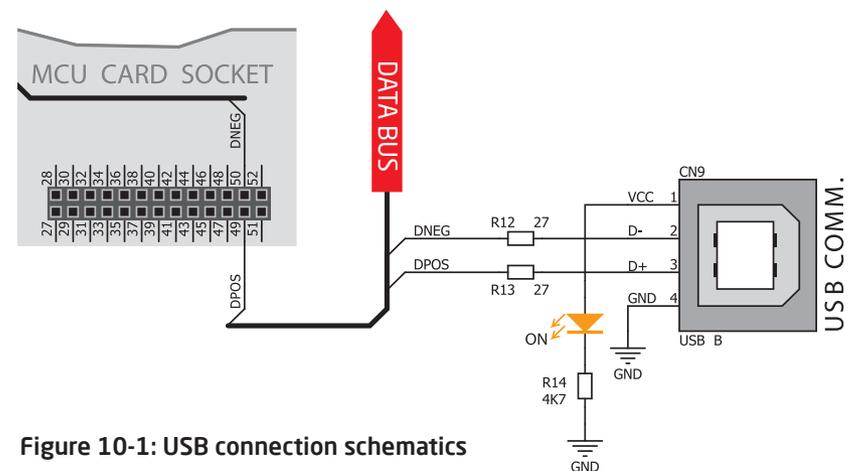
Figure 10-1: USB connection schematics
