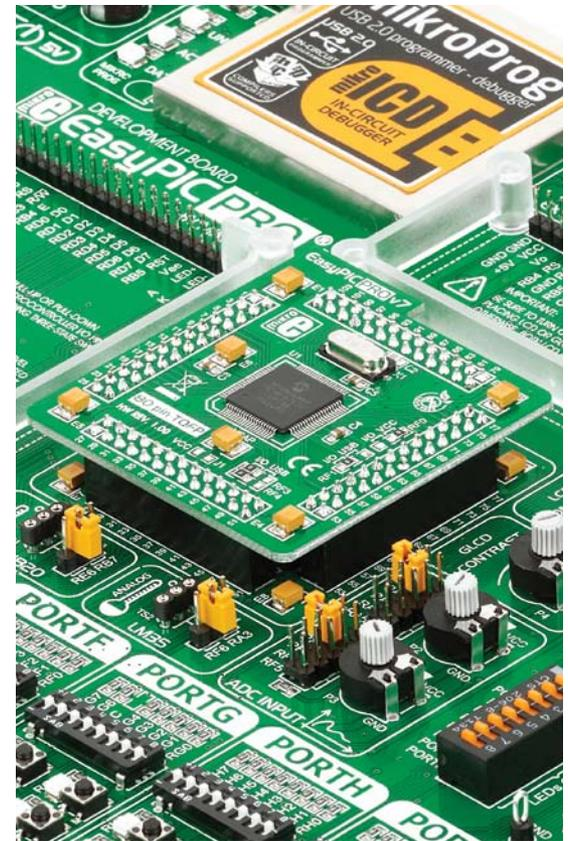
**3** Figure 4-5: Properly placed MCU card will have equally leveled pins.
