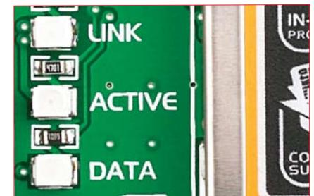
Three LEDs indicate specific programmer operation. **Link** LED lights up when USB link is established with your PC, **Active** LED lights up when programmer is active. **Data** is on when data is being transferred between the programmer and PC software (compiler or mikroProg Suite™ for PIC®).
