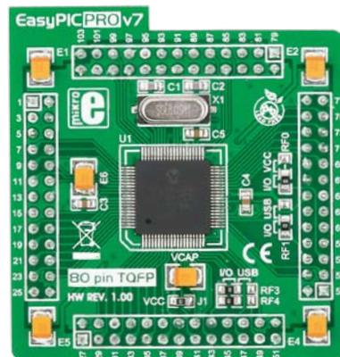
2 Figure 4-3: Standard 80-pin MCU card with **PIC18F8520**.
