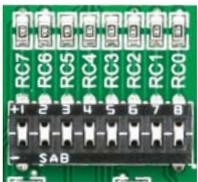
Tri-state DIP switches, like **SW3** on **Figure 6-2**, are used to enable 4K7 pull-up or pull-down resistor on any desired port pin. Each of those switches has three states:
