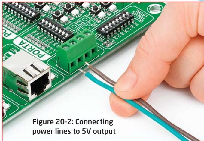
Figure 20-2: Connecting power lines to 5V output
