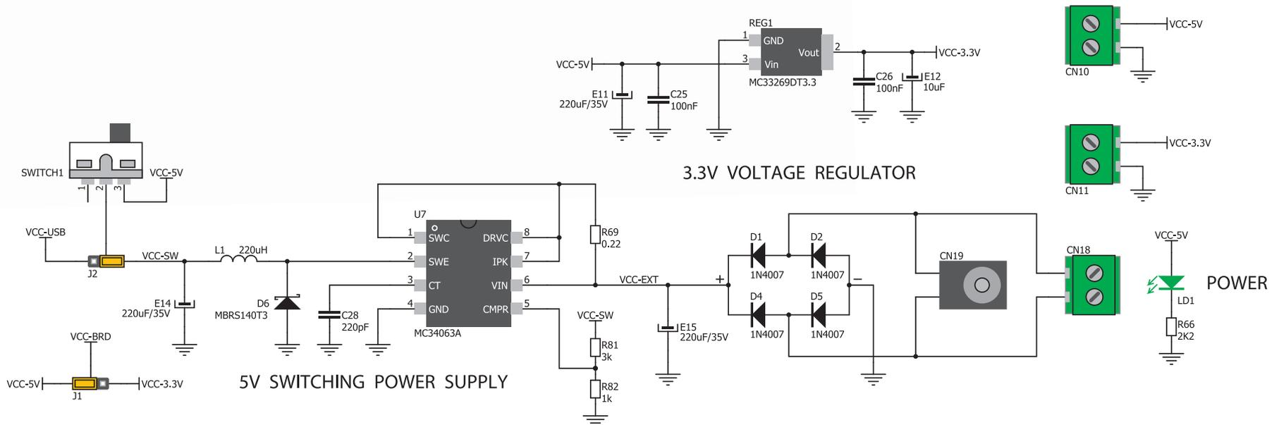
Figure 3-2: Dual power supply unit schematics
