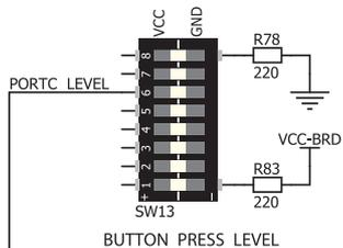
Button press level tri-state DIP switch is used to determine what logic state will push buttons be connected to when pressed
