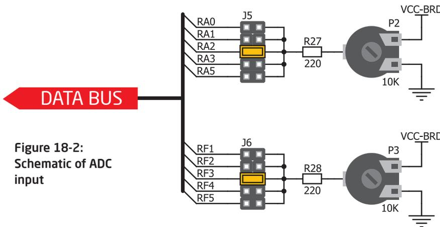
Figure 18-2: Schematic of ADC input
