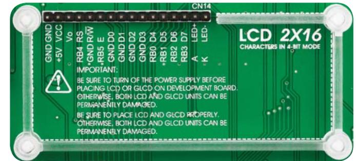
Figure 12-1: On-board LCD 2x16 display connector
