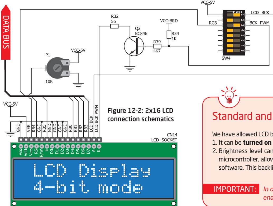
Figure 12-2: 2x16 LCD connection schematics
