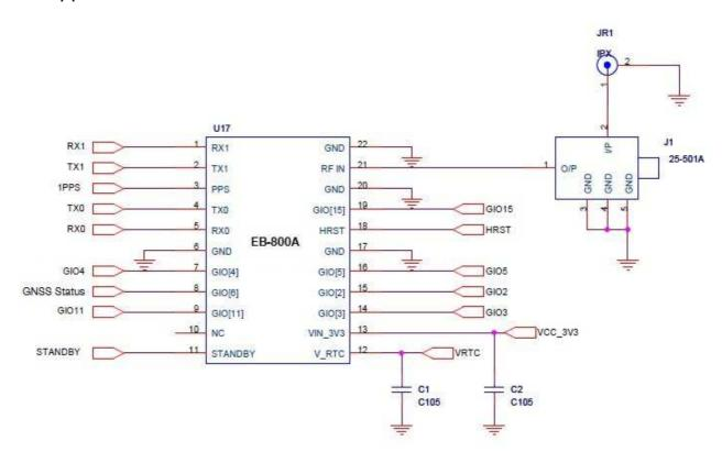
[Note1]: GPIO[6] (pin#8) can be used as GPS / Glonass position fix indicator.
