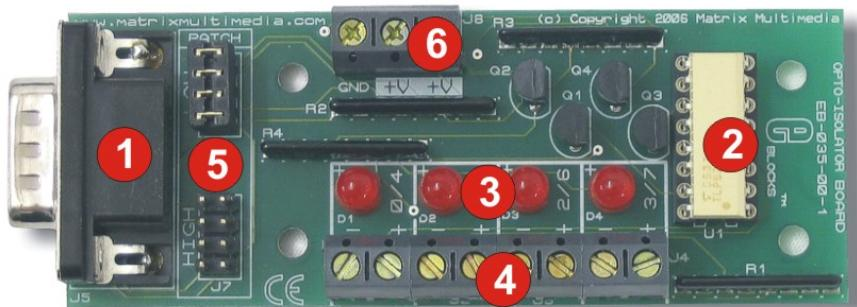
NB. Please ensure the mode selection jumpers are arranged on the board with the metal connection strips positioned horizontally.
