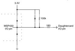
The I/O pins can sink or source approximately 10mA maximum, with the actual current determined by the pin impedance, the series resistor, and the load resistance. An LED can be directly connected between an I/O pin and 3.3V or ground without exceeded the MSP430 current limits.
