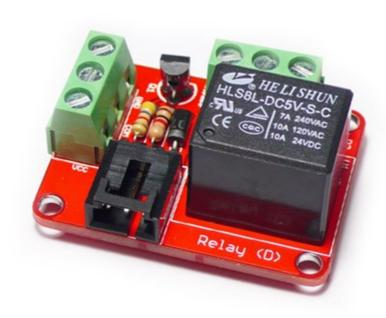
This Brick uses an HLS8L relay module to control high-voltage electrical devices. (maximum 240VAC, 7A; 120VAC 10A; 24VDC 10A).
